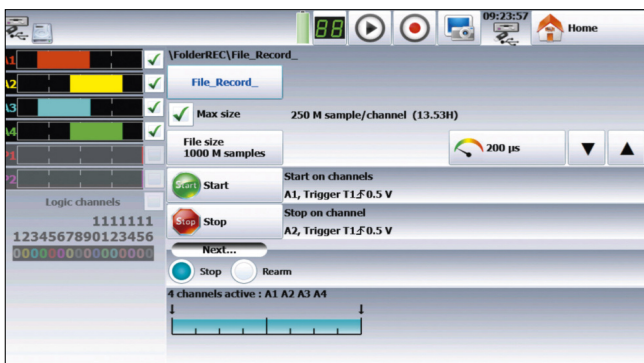
Trigger: several type of trigger, one channel, on a level, slope, several channels or combined conditions.
