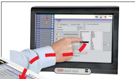
With Virtual Network Computing software, you remote control your DAS801 from a computer or a tablet.
